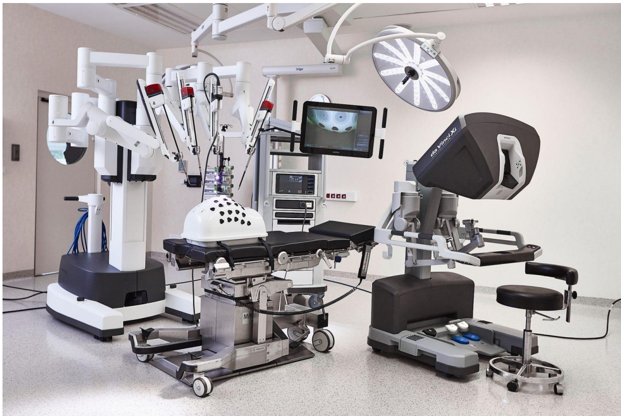
Figure 1: The da Vinci with attached EndoWrists
