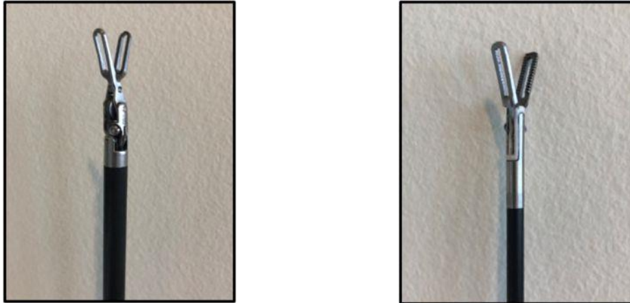
Figure 5: EndoWrist forceps vs. Traditional manual forceps
