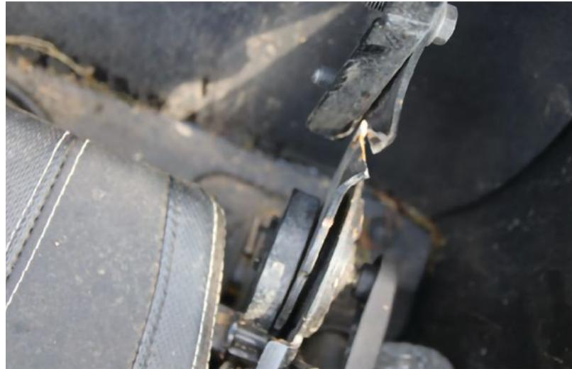
Additionally, the seatback is attached by inadequate screws that can readily break free from their mounting points during impact, allowing the seat to partially separate and move vertically, contributing to occupant ejection. The small screws are attached into the plastic of the seatback. This risk is further exacerbated by the aforementioned lack of a seatbelt pretensioner to keep the occupant further restrained.
